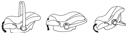
Face the restraint, push the red button on each side of handle, rotate and release red button to desired position until hearing a "click". There are five positions of rotating.
